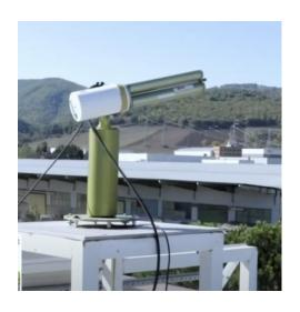
Photometer points at Sun and measures radiance at different wavelengths.
